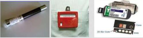
The image shows three types of dosimeters: a cylindrical ionization chamber, a red film badge, and a black TLD badge with a digital display.
