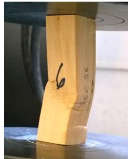
Figure 3. Test specimen showing flexo-compression
