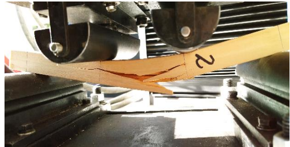
Figure 6. Pure flexion tests
