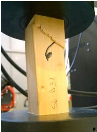
Figure 4. Compression test specimen of 50 mm x 50 mm x 150 mm
