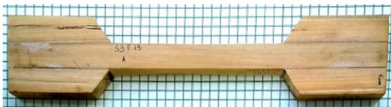
Figure 1. Tensile test specimen
