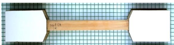
Figure 2. Tensile test specimen with joint cover
