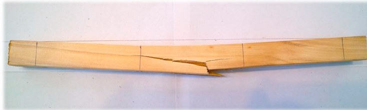
Fig. 7. Pure bending tested specimen.
