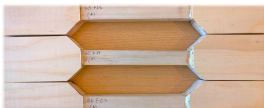
Fig. 2. Specimen for tensile test.
